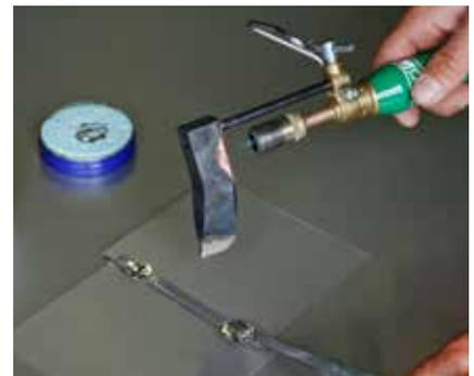
Press the solder rod until the solder has cooled off and joins the metals, lift the soldering bit for faster cooling
