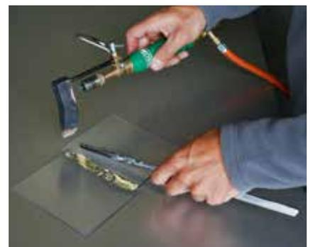
You can see if solder has cooled off enough when the solder surface tarnishes.
