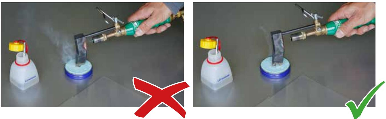
a. Soldering bit too hot: heavy smoke formation when dipping the soldering bit into salmiak stone (ammonium chloride / soldering stone)
