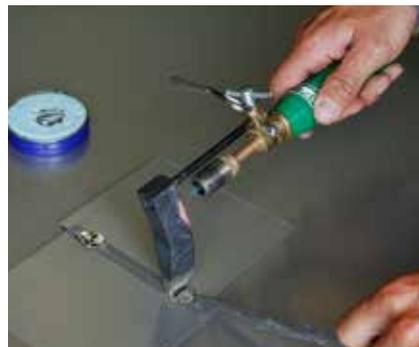
Transfer solder to the tack spot and press the solder bar to the tack spot
